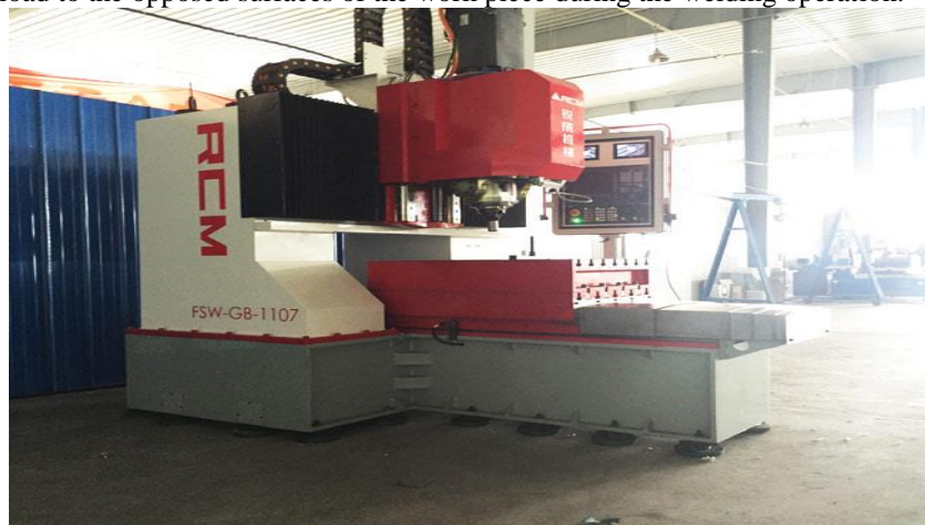
Fig.3. Experimental set up of FSW in BARC
