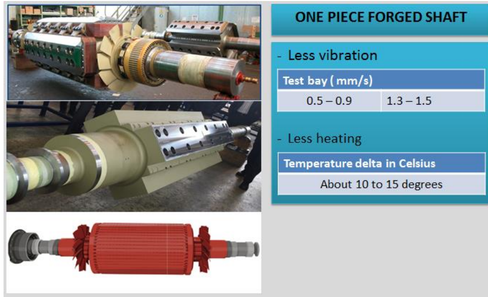
Figure 6: Rotor construction
