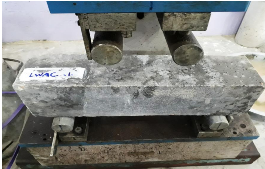
Fig.2 : Lightweight Aggregate Concrete For Flexural Strength Test ( Third Point Loading)
