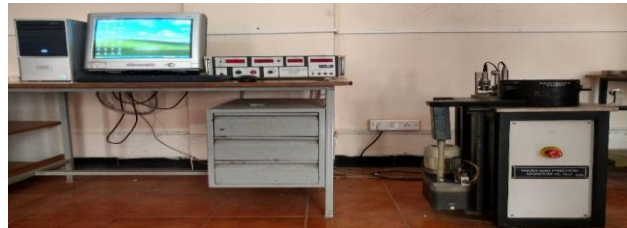
Fig. 2: Pin-on-disc Setup and Wear Monitor
