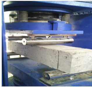
Figure.5 Flexure Strength Test
