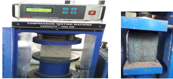
Figure.3 Setup for Compressive strength
