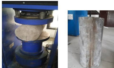
Figure.4 Setup for Split Tensile Strength
